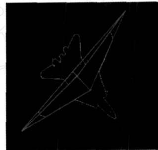
图 11 特征点提取 Fig. 11 Extraction of feature points
